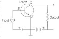
resistance path. The weak input signal is applied across the forward biased junction, and the output signal is taken across the reverse biased junction.
