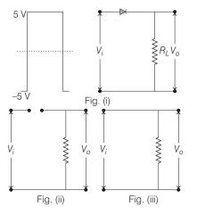
For  $V_i < 0$ , the diode is reverse biased and hence offer infinite resistance, so circuit would be like as shown in Fig. (ii) and  $V_o = 0$ .
